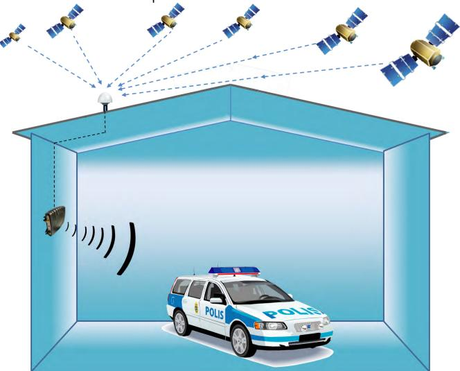
To use GNSS satellite devices inside your building you will need a repeater system to transfer the outdoor signals to inside. A repeater is a device that relays GNSS signals to any indoor location that isn't normally reachable.
